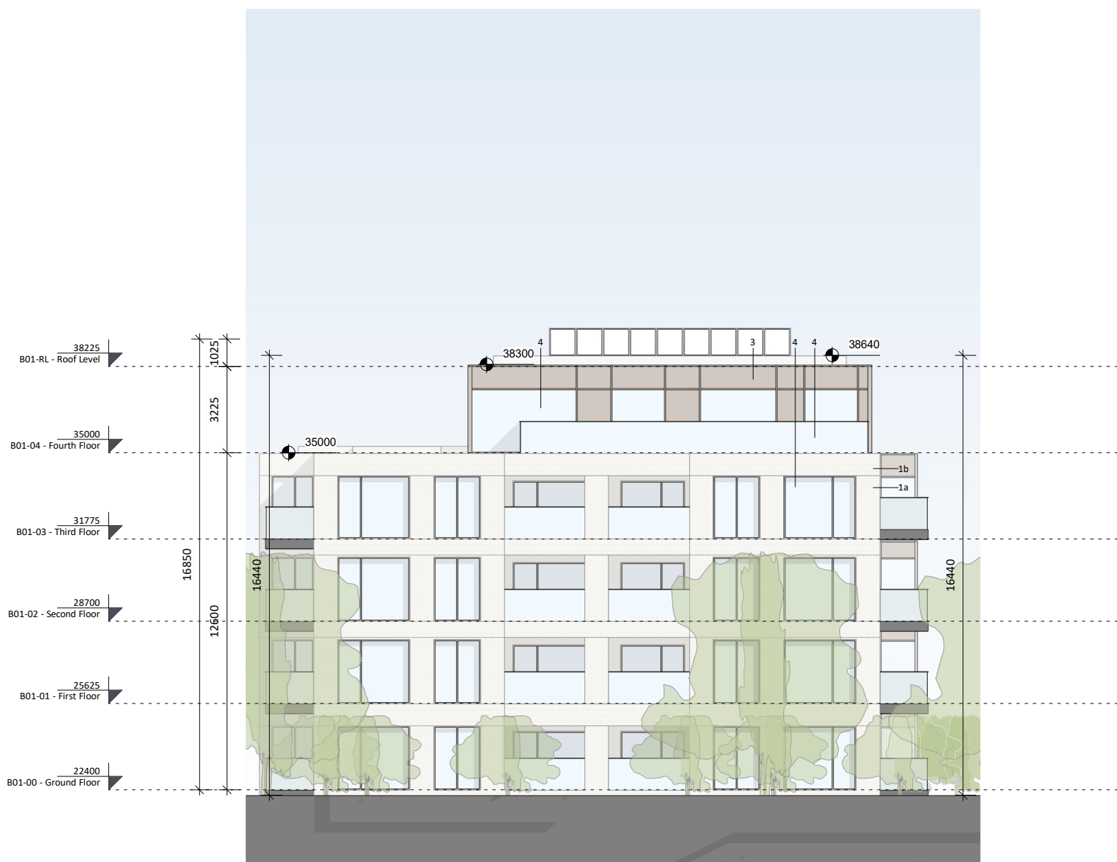
② Block 01 South Elevation 1 : 200
